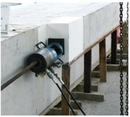
Concrete with GFRP dowels & post-tensioned steel bar
