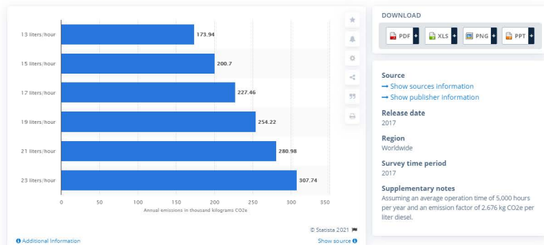
Average carbon dioxide (CO2) emissions of diesel-electric rubber-tired gantry (RTG) cranes at ports worldwide in 2017, by consumption (in 1,000 kilograms CO2e per year)
