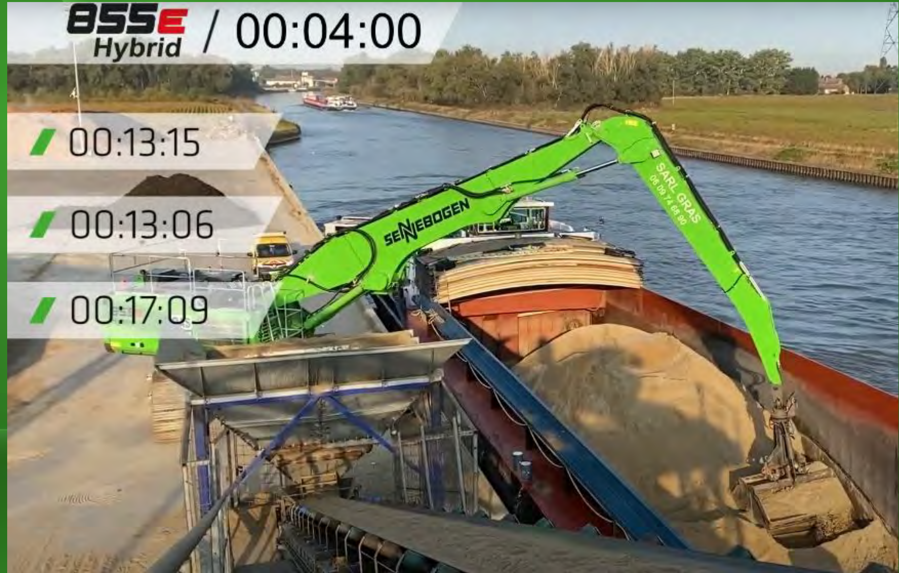
SENNEBOGEN 855 E Hybrid | Sand offloading in average under 20 sec cycles
