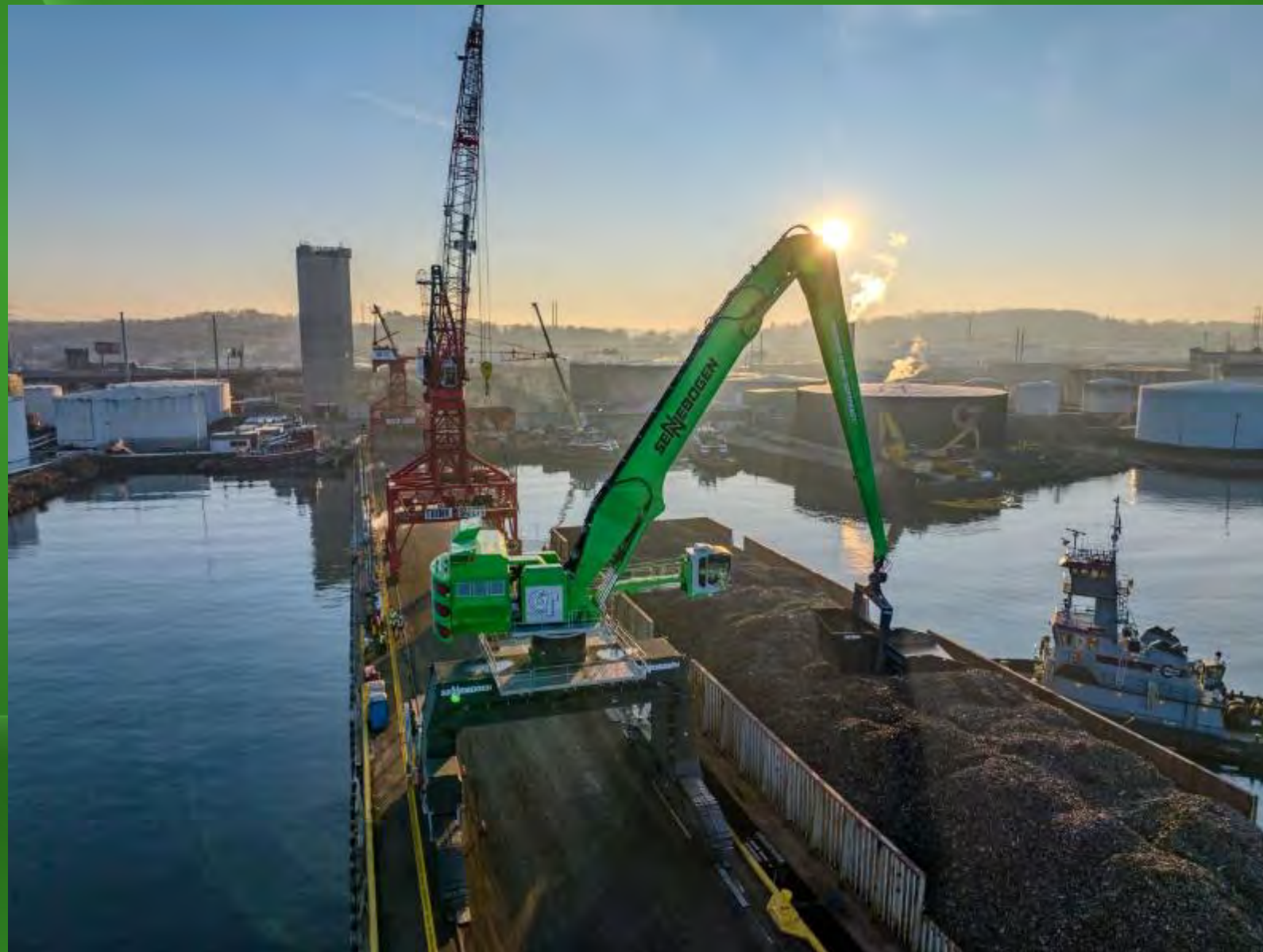
SENNEBOGEN 895 E on Rail Gantry | 895 with 26m 3 skip pan loading shredded scrap
