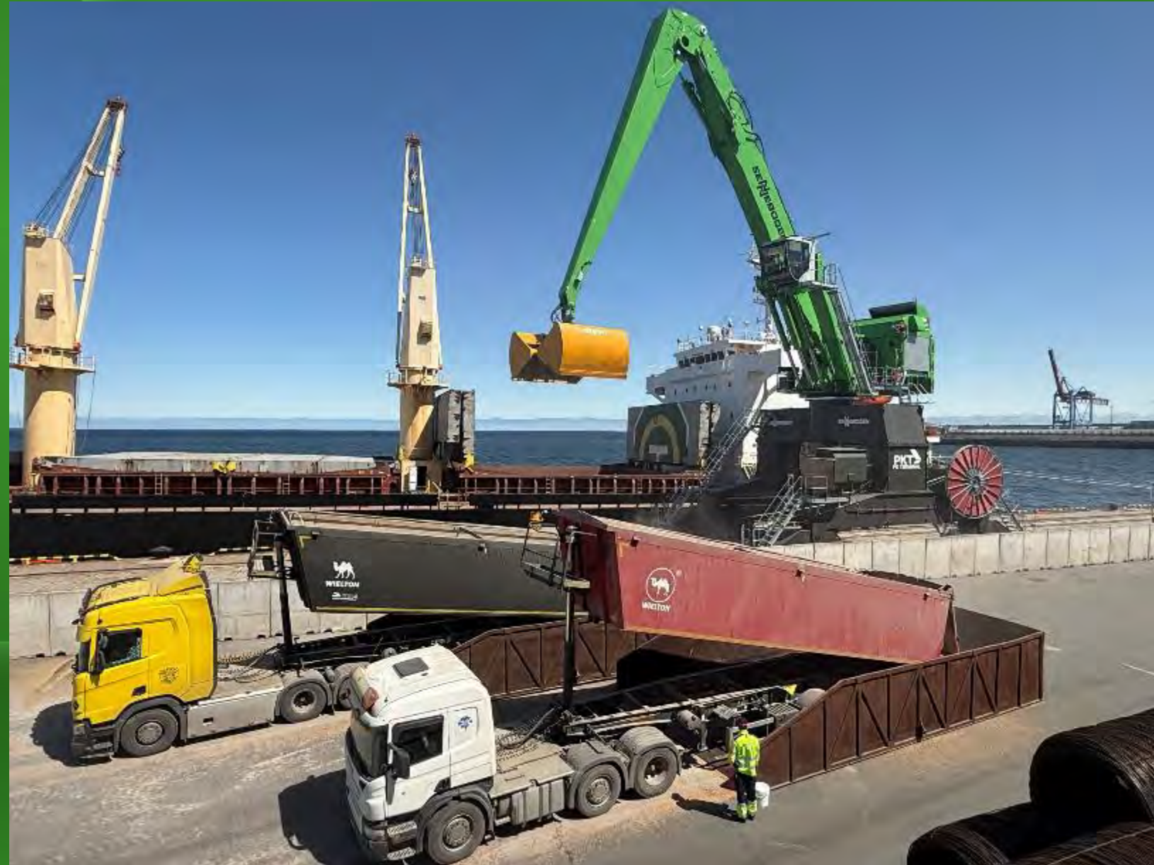
SENNEBOGEN 885 E on Rail Gantry | Bulk Handling between Inland Ships and Freight Trains
