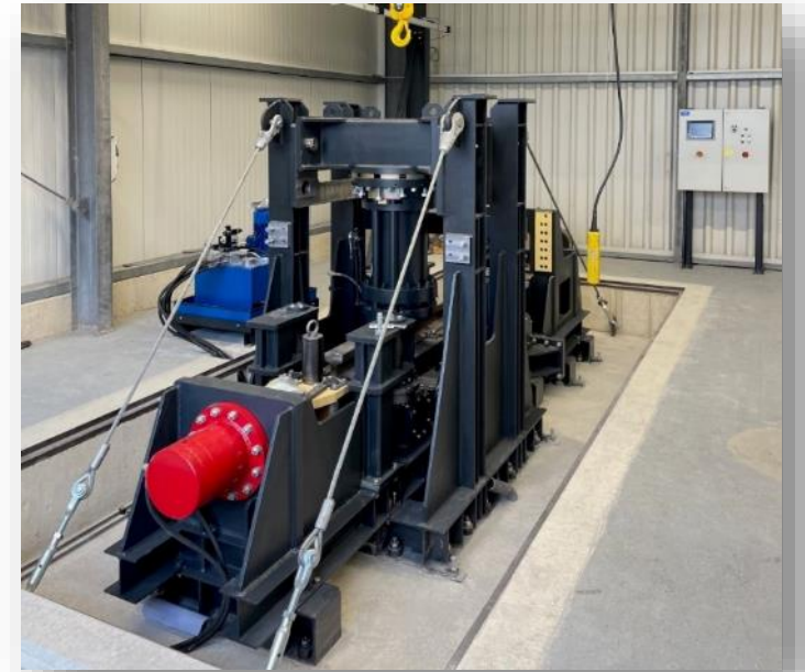
Dynamic storm brake test rig Holding forces over 1000 kN
