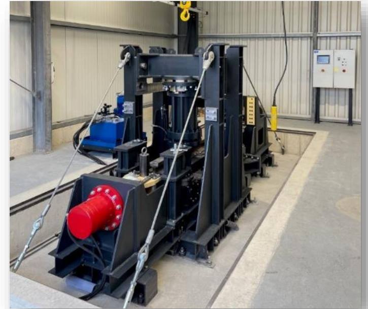
Dynamic storm brake test rig Holding forces over 1000 kN
