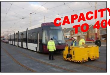
**COMPACT ROAD-RAIL SHUNTER (W 2200 mm** x L 1830 mm), able to transversally enter/exit from track side, without any maneuvering, in a quick and easy movement.
