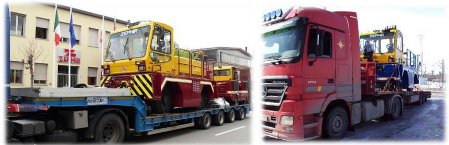
The LOCOTRACTOR is easily relocated to another terminal, by truck or freight wagon, as the maximum width is standard at 2.5 metres and they have a low gross vehicle weight.
