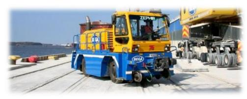
Rail wear and track maintenance costs are also reduced, due to the lighter vehicle weight, traction by the rubber wheels and the specially designed rail guide wheels of the LOCOTRACTOR.
