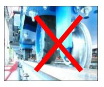
This simple configuration is producing a lot of dangerous situations since the rail wheel which should be guiding the vehicle can easily loose completely the contact with the rail track.
