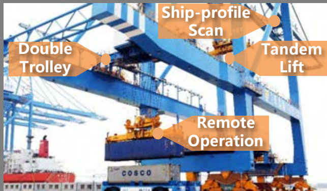
Automated STS Crane
