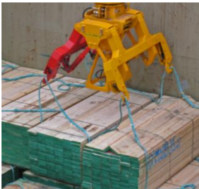
Timber pack traverse
