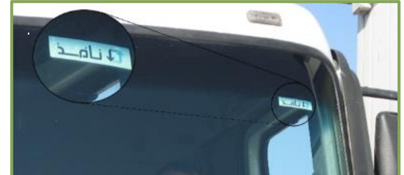
Truck eID Secure RFID tags, Trailer/Chassis eSeals
